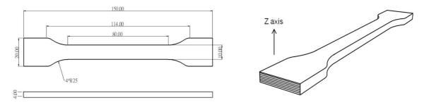
FLEXURAL TESTING SPECIMEN ISO 178, GB/T 9341
